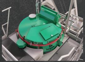
**PDL MINI-MAX** is a compact production line for small customers expecting high manufacture quality. It is the smallest of all production lines that we have in our offer, a perfect choice for companies seated at a considerable distance from concrete plants. The production line is composed of the stationary PHS Mini-Max machine, the RMT 600/400 mixer, aggregate feeder and a concrete mix belt feeder.
