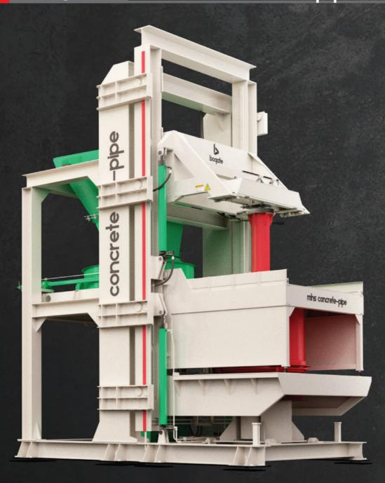
MHS Concrete-Pipe is a fully automated stationary hydraulic machine used to produce concrete manhole rings and pipes. It is an excellent choice for those customers who expect high production capacity and fully-automated processes. The machine is controlled through the fail-safe Mitsubishi FX controller, which guarantees smooth production and precise control of all parameters of the machine.
